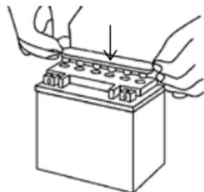
**IMPORTANT:** Never remove the cap strip or add water or electrolyte to the battery.
