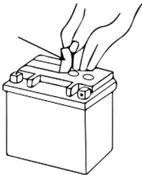
**2.1.1** Remove foil strip which runs across the top of the battery filling reservoir.
