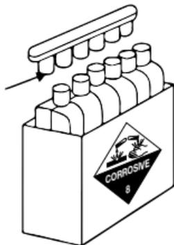
**2.1.3** Place electrolyte container, sealed top of the cells down, into the filler ports of the battery and push down to break the seals. Ensure the electrolyte container is kept in an upright position during this process.
