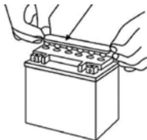
**2.1.7** Charge the battery in line with the following: 0.1CA x (5-10)Hr OR 0.5CA x (0.5-1)Hr
